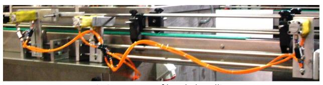
Penumatic Separators of bottle handling system
