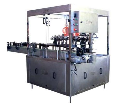
Rinsing unit neck holding bottle grippers & output Star
