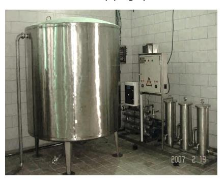
Stainless steel pre-treatment tank and UV pipe rows, buster pump and Micro filter cylinders
