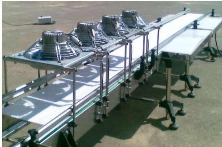
The wide width Conveyor equipped with drier fans
