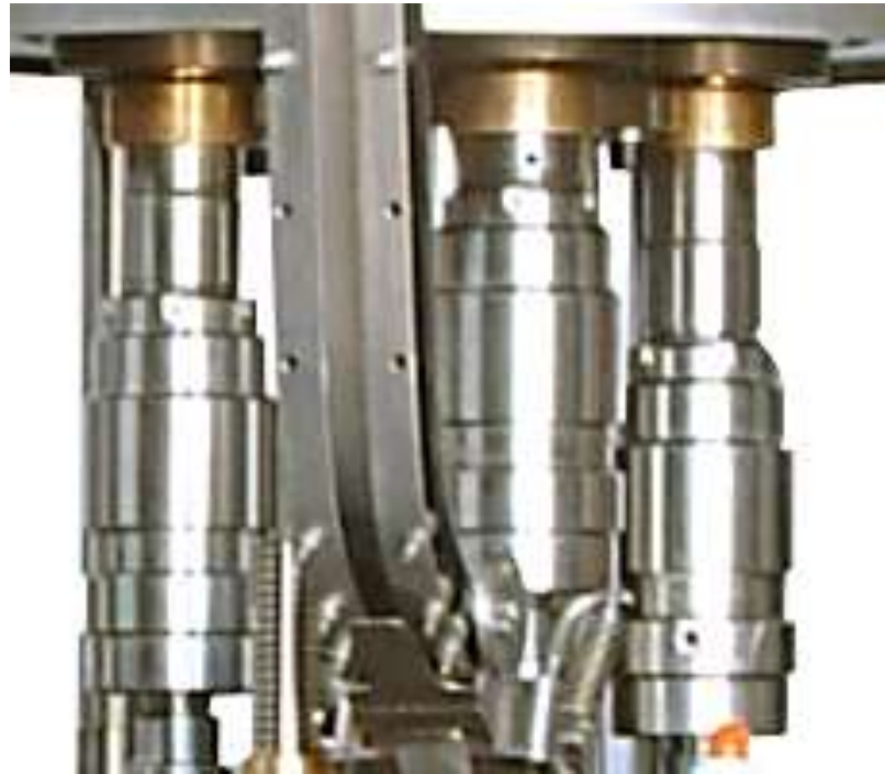
Capping Heads equipped with Magnetic Clutch
