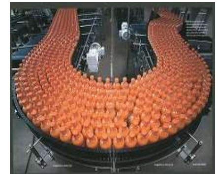
U form Mass conveying system
