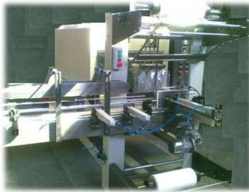
Shrink pack machine equipped with bottles sorting system
