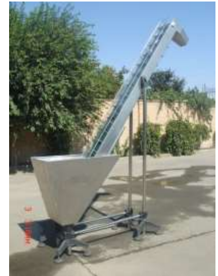
Hopper conveyor with reservoir
