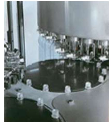
Filler`s stainless steel ring bowl & Bottle movement neck handling system with star discs and external guides
