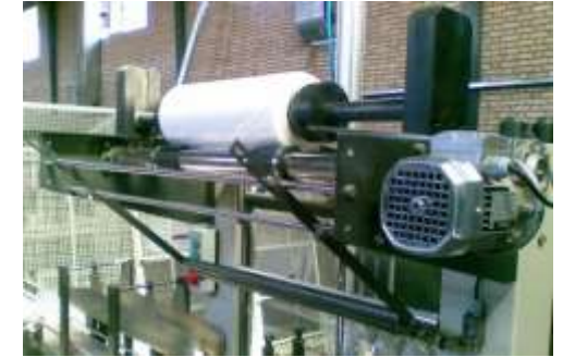
Plastic Cover roll feeding system
