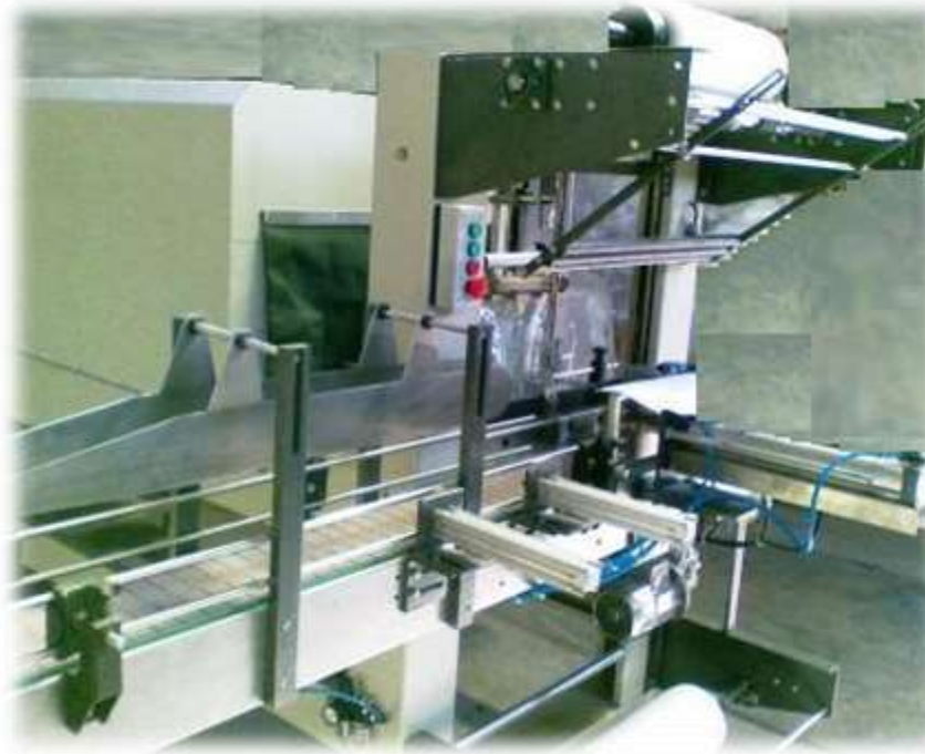
Shrink pack machine equipped with bottles sorting system
